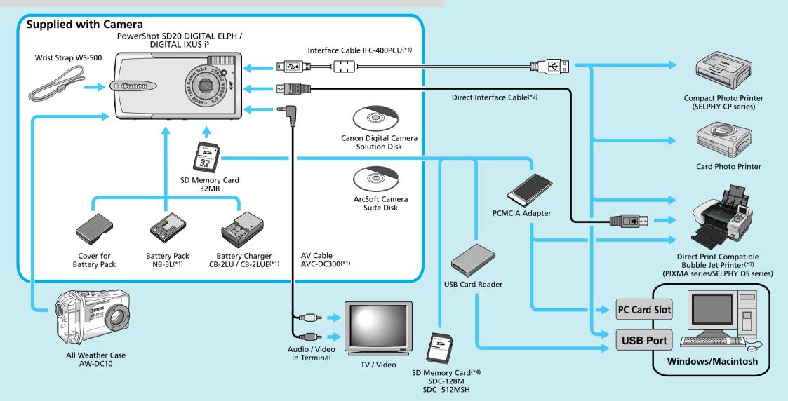
This camera can also be connected to the Card Photo printers.
