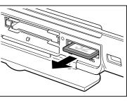
Do not remove memory cards or turn the printer off while the indicator lamp is blinking.
