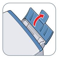
**3** Place a stack of paper (print side up) in the multi-purpose tray ① and adjust the paper guide (A) to the width of the stack ②. Make sure the stack does not exceed the paper limit mark (B).
