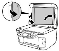
(2) Remove both the film guides for film strip or slides from the rear of the FAU Protective Sheet.
