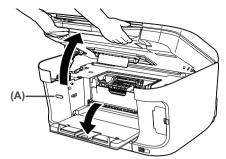
(A) Press the Open Button to open the Paper Output Tray if it does not open automatically.
