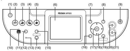
(1) [ON/OFF] Turns the machine ON and OFF. Before turning ON the machine, make sure the Document Cover is closed.
