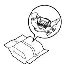
6 Remove the protective cap (A) from the Print Head.
