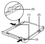
Do not load higher than the Load Limit Mark (A).
