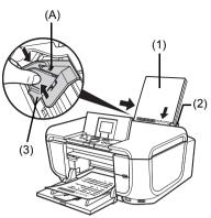
Do not load higher than the Load Limit Mark (A).
