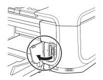
3 Insert one and only one memory card into the Card Slot.
