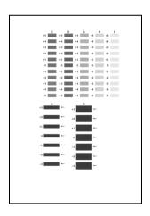
13 Look at the printout. From the patterns, select the most even patterns for each column and input their numbers. Press the **OK** button. In the same way in step 9, input the numbers.
