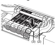
Make sure the position of the tank matches the label.
