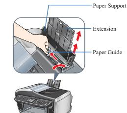
**2** Load a few sheets of letter- or A4-size paper into the Auto Sheet Feeder, align the paper with the right side of the Cover Guide, then slide the Paper Guide toward the left edge of the paper.
