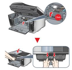
**A** IMPORTANT For safety, always firmly grip the areas illustrated when closing the Scanning Unit (Printer Cover).
