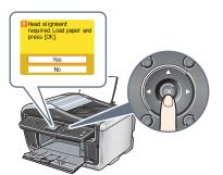
The pattern is printed. And Print Head is aligned automatically.
