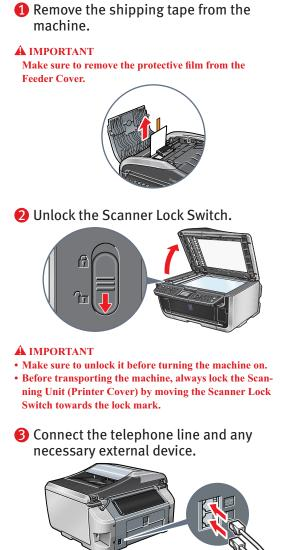
Connect the telephone line cord to the wall jack. You can connect an external device (telephone or answering machine) if necessary
