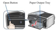
Open the Scanning Unit (Printer Cover) until it locks into place. The Print Head Holder moves to the center.
