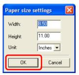
When Custom is selected, a dialog allowing you to specify the dimensions will appear. After selecting the units of choice, input the dimensions and click the [OK] button.
