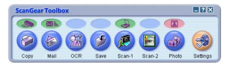
The symbols in this space show which scanner button is assigned to which Toolbox function. The examples above indicate the following assignments.
