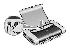
**Important** • Before unplugging the power cord, turn off the printer and ensure that the green lamp has gone out.
