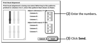
**Note** If it is difficult to pick up the best pattern on Column F, pick the setting that produces the least noticeable vertical white stripes.
