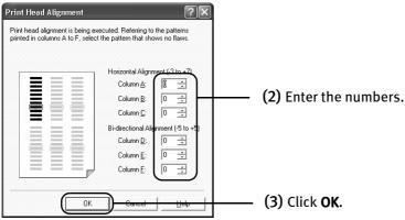
**Note** If it is difficult to pick up the best pattern on Column F, pick the setting that produces the least noticeable vertical white stripes.
