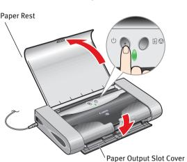
IMPORTANT: Do not open the cover before the printer has finished initializing. Wait until the POWER lamp remains fully lit.
