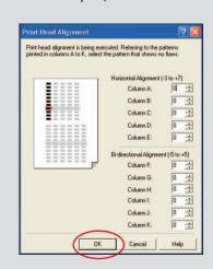
Click **OK** to exit the Maintenance tab. Print head alignment is now complete.
