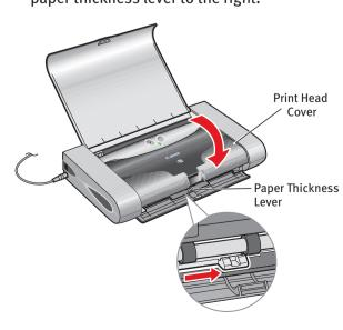
NOTE: The printer will perform a print head cleaning after the cover is closed. Wait until the process is complete before proceeding.
