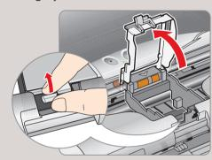
Place the print head into the holder, by aligning the
