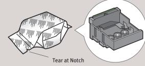
2 Remove the protective cap from the print head.
