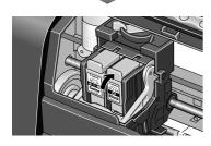
(2) Press on the tab until the ink tank snaps firmly into place
