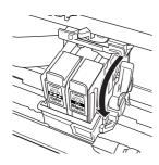
**6** Lock the BJ Cartridge into place by lowering the lever.
