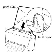
**5** Press the paper guide and slide it against the left side of the stack of paper.
