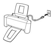
**1** Plug the printer in. Do NOT turn on the computer yet.
