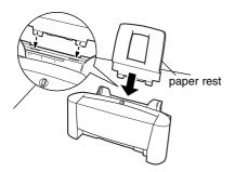
**3** Attach the paper rest to the sheet feeder.
