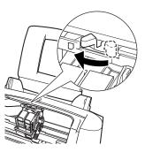
For regular paper and other media with a left position in the table (see "Load Limit and Paper Thickness Lever Position" on page 4).
