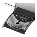
•If you use a SmartMedia card, hold the exposed portion of the memory card with your fingers to remove the memory card.
