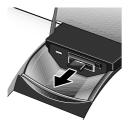
•If you use an SD card or MultiMedia card, hold the exposed portion of the memory card with your fingers to remove the memory card.
