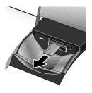
• If you use a Memory Stick, hold the exposed portion of the memory card with your fingers to remove the memory card.
