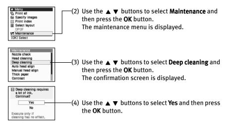
**Important** The process takes one or two minutes to complete, so simply wait until the **Power** lamp stops flashing.
