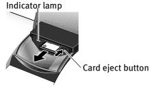
•If you use CompactFlash (CF) card or Microdrive, press the card eject button to remove the card.
