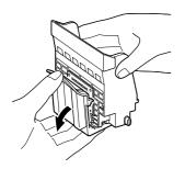
**6** Remove the protective cap from the print head.
