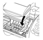
**8** Lock the print head into place by lowering the lever.
