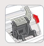
Gently slide the print head into the holder. The print head will rest at a slight angle. Do not press it down.
