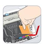
4 Insert the remaining three ink tanks into their assigned slots.
