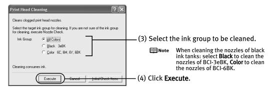
**Print Head Cleaning** starts when the **POWER** lamp starts blinking.
