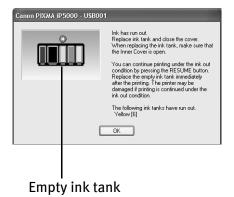
The ink tank with [X] symbol is out of ink. Replace with a new ink tank.
