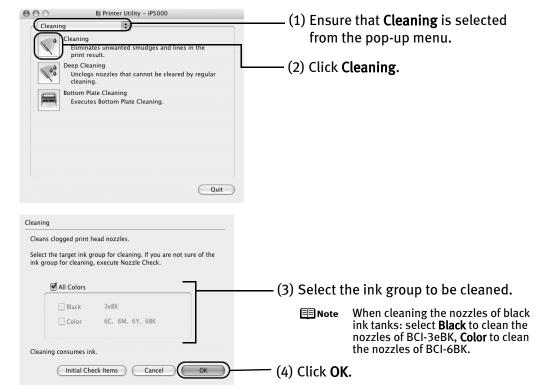
**Print Head Cleaning** starts when the **POWER** lamp starts blinking.
