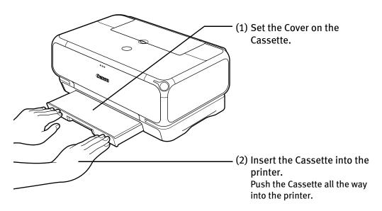
Note If the Cassette has been extended to accommodate paper sizes larger than 5" x 7", the front edge of the cassette will extend beyond the front of the printer.
