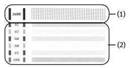
(1) If lines of this pattern are missing, the "Black" print head nozzle needs cleaning.
