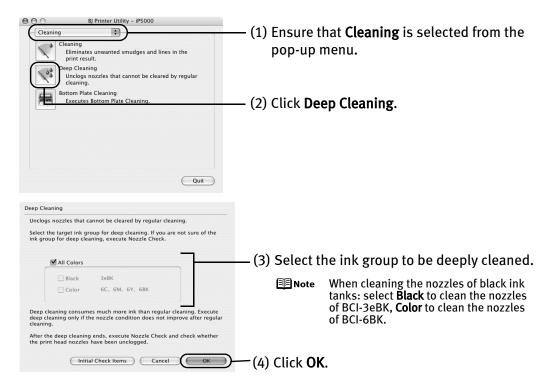
Print Head Deep Cleaning starts when the POWER lamp starts blinking.
