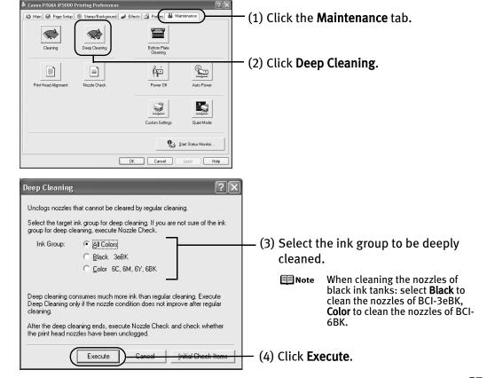
**Print Head Deep Cleaning** starts when the **POWER** lamp starts blinking.
