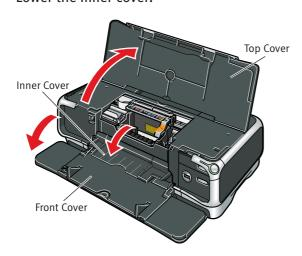
The print head holder automatically moves to the center. Remove the protective tape.
