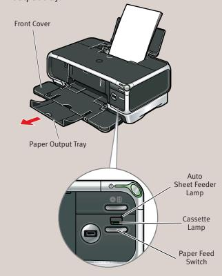
**NOTE:** When feeding paper from the cassette, press the paper feed switch so that the cassette lamp turns on.
