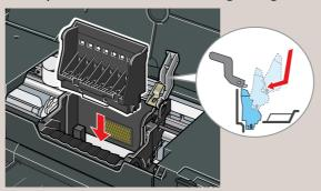
**5** Lower the print head lock lever and press it down until it clicks into place.
