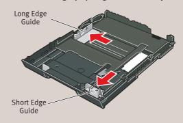
5 Load paper so that the top right corner touches the inside corner of the cassette. Adjust paper guides to the edges of paper.
