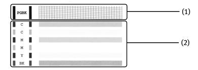
(1) If line of this pattern are missing, the "Black" print head nozzle needs cleaning.
