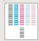
For each color on the test printout, enter the number in the Print Head Alignment window that corresponds with the smoothest looking test pattern.
