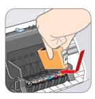
4 Insert the remaining five ink tanks into their assigned slots.
