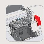
Gently slide the printhead into the holder. The printhead will rest at a slight angle. Do not press it down.
