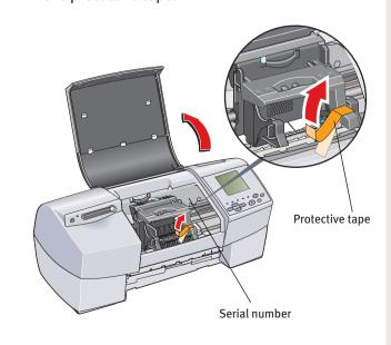
Write down the serial number located to the right of the printhead. You will need this later to register the product. 3 Install the Printhead
