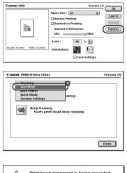
Print head alignment is being executed. Alignment entails printing, so do the following: Ready the printer (connect the cable and turn the power on), move the printer's paper thickness iever to the left, and load a sheet of plain paper in the sheet feeder. Do you want to print head alignment patterns?
