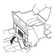
6 Remove the protective cap from the print head.
