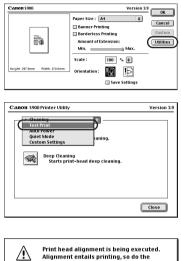
Alignment entails printing, so do the following: Ready the printer (connect the cable and turn the power on), move the printer's paper thickness lever to the left, and load a sheet of plain paper in the sheet feeder. Do you want to print head alignment patterns?
