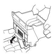
**6** Remove the protective cap from the print head.
