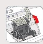
4 Slide the printhead into the holder. The printhead will rest at a slight angle.
