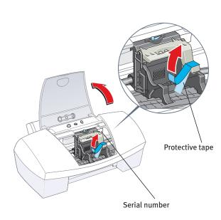
Write down the serial number located to the right of the printhead. You will need this later to register the product.
