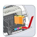
4 Insert the remaining three ink tanks into their assigned slots.
