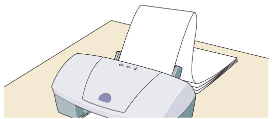
Place the printer where the printed banner output can hang over the edge of the table.
