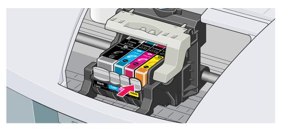
Do not touch the lock lever; remove only the ink tank.
