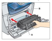
**5** Hold the cartridge so that the instructions (**A**) and the arrow (**B**) are facing up, and insert it in the machine horizontally as far as it will go.
