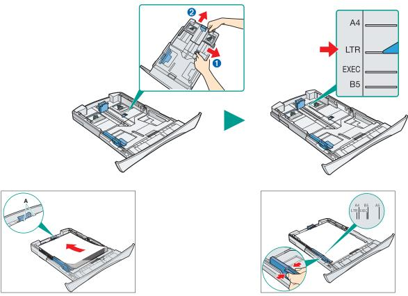
**5** Load the paper into the cassette. Make sure the paper stack sits below the hooks (**A**).
