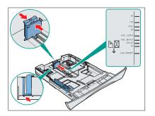
**4** Pinch and slide the rear paper end guide to match the size of paper.
