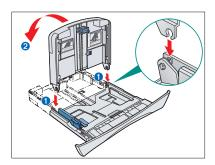
**3** Attach the extension to the cassette. The slots • are keyed and must be inserted at a 90° angle. Once inserted, fold the extension as shown ②.
