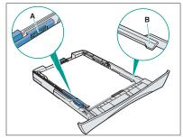
**7** Even out the edges of the paper stack. Make sure the height of the stack does not exceed the limit marks (A) and that the side edges of the stack are below the hooks (B).
