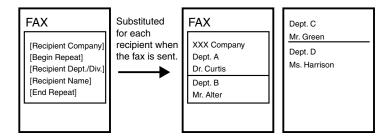
In addition to the [Sender Information] and [Recipient Information] fields, you can also insert [Sheets to Send], [Remark], and [Comment] fields on the cover sheet. When the fax is sent, the number of sheets to send as a fax specified in the fax driver is inserted in the [Sheets to Send] field, information specified in the fax driver, such as [Urgent] or [Confidential] is inserted in the [Remark] field, and comments specified in the fax driver are entered in the [Comment] field.
