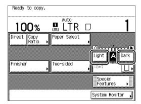
Press [Light] to move the indicator to the left to make the exposure lighter, or press [Dark] to move it to the right to make the exposure darker.
