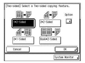
To set the orientation of the two-sided copies, press [Option] → select the type of two-sided orientation → press [Done].
