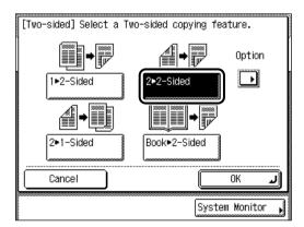
To set the orientation of the originals and the copies, press [Option] → select the type of two-sided orientation for the originals and the copies  $\rightarrow$  press [Done].
