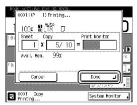
If the job displayed on the touch panel display is from a function other than the Copy function, press [Done] → COPY) to display the Copy Basic Features screen.
