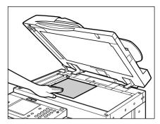
The surface of the original that you want to copy must be placed face down. Align the top edge of your original with the back edge of the platen glass (by the arrow in the top left corner).
