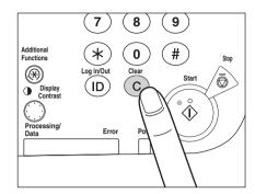
Press ① - ⑨ (numeric keys) to enter the desired copy quantity (1 to 99).
