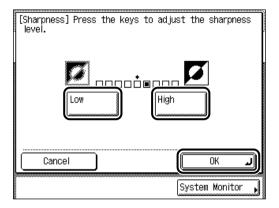
To copy text or lines clearly, the setting should be towards [High]. To copy originals containing printed images or other halftones, the setting should be towards [Low].
