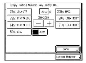
The selected mode is set, the display returns to the Copy Basic Features screen, and the copy ratio generated by the machine is displayed.
