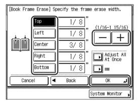
To return to the screen for setting the same width for all four borders, press [Adjust All At Once].
