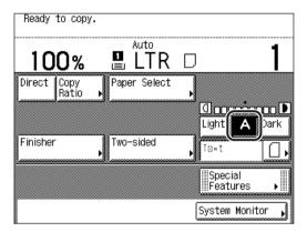
The machine automatically adjusts the copy exposure to the level best suited to the quality of the original.
