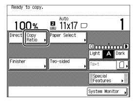
2 To reduce the original image, select a preset reduction ratio. To enlarge the original image, select a preset enlargement ratio. Following your selection, press [Done].
