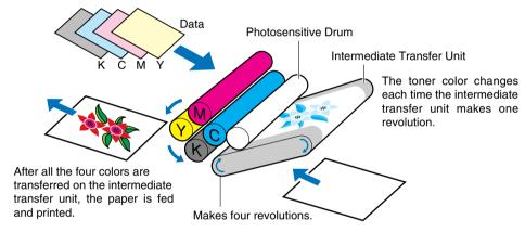
When data in all four colors is transferred onto paper, the paper goes through the fuser unit and is output.
