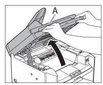
3. Open the toner cover (B), using the knob which covers over on dent (A).
