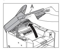
Open the toner cover (B), using the knob which covers over on dent (A).
