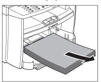
12. Remove the paper cassette by lifting up the front-end of the paper cassette and pulling it forward.
