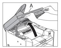
2. Open the toner cover (B), using the knob which covers over on dent (A).
