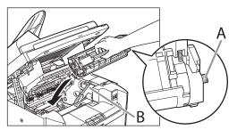
9. Push the toner cartridge to make sure it is properly set in the machine.
