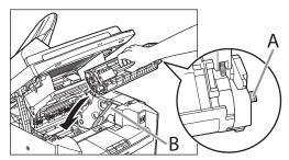
9. Push down the toner cartridge to make sure it is properly set in the machine.
