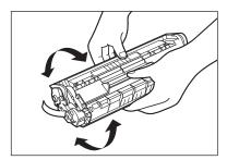
6. Hold the toner cartridge with one hand, and pull the seal completely out.
