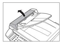
3. Clean the rollers (A) inside the ADF with a cloth dampened with water. Then wipe the area with a soft, dry cloth.
