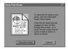
When you click the **Clean Print Heads** button, the printer automatically cleans the print heads.
