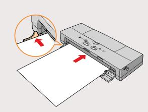
4 Hold the sheet for about 2 seconds; it will automatically feed partially into the printer.
