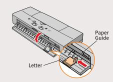
3 With the side you want to print on facing up, insert a sheet of paper into the printer until it stops.
