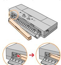
4 Press on the right side of the battery pack to lock it in place.
