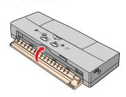
**NOTE:** You must install the battery pack. If the battery pack is not installed when you turn on the printer, the CHARGE/ERROR lamp will light orange and the printer will beep six times.
