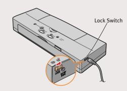
**NOTE:** When the power lock switch is to the left, you cannot turn the printer on.
