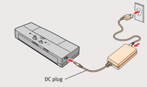
**NOTE:** The green CHARGE/ERROR light stays on until the battery pack is completely charged (approximately 4 to 6 hours).
