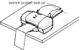
As the sheets print, allow the printed sheets to hang over the edge of the desk or work table.
