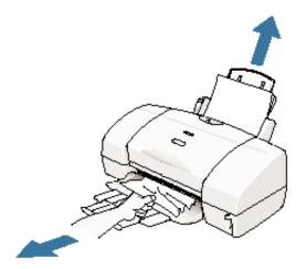
If the paper tears off inside the printer, turn off the printer. Open the printer's cover, and remove the paper left inside the printer.
