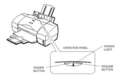
POWER button Press to switch the printer on and off.
