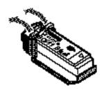
6. Carefully slide the new ink tank into the empty slot on the BJ cartridge.
