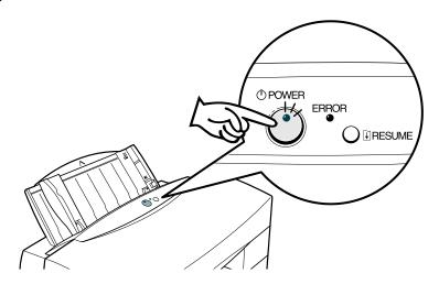
If no BJ Cartridges are installed, the **POWER** lamp flashes, the **ERROR** lamp lights, and the printer beeps four times. You must install the BJ Cartridges and ink tanks. (\$\sigma\$ 27, 33)
