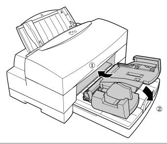
Push the paper output receiver into the printer until it locks in place. Make sure the paper output receiver is inserted completely inside the printer.
