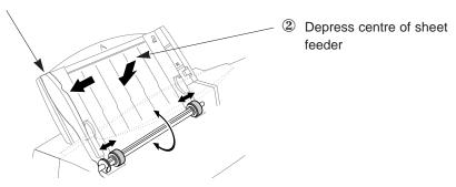
3 Rotate the axis of the feed roller as you clean the grey bands on either end.
