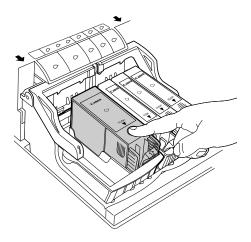
${\bf 6}$   $\,$  Install the Ink Optimizer Tank BCI-8WF in the black BJ Cartridge.
