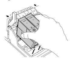
$\mathbf{6}$  Unwrap the new BJ Cartridge and remove the orange protective cap.
