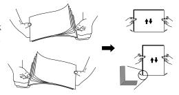
With the printing sides (glossy sides) facing up, align the sheets with the right side of the sheet feeder and insert them straight into the paper feed slot until they stop. Always load them vertically.
