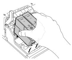
6 Store the Black BJ Cartridge BC-80 in the left slot of the BJ Cartridge Container SB-80.
