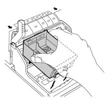
**Q** Lower the cartridge lock lever to lock the BJ Cartridge in place.
