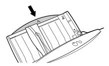
**9** Raise and lock the envelope guides on both sides of the sheet feeder.
