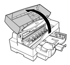
3 Press the **REPLACE** button. The cartridge holder moves to the left side of the printer.
