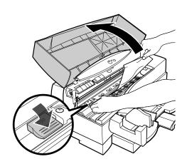
Remove the paper stack from the sheet feeder and fan it to remove static cling then load it in the sheet feeder again.
