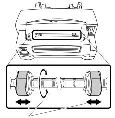
As you rotate the feed roller on its axis, move the cloth from side to side to clean the grey bands on either end of the feed roler.
