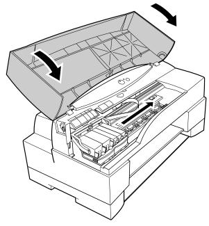
After you close the top cover, you will hear the cartridge holder return to the home position. It will take a few moments for this movement to complete and for the printer to clean the print heads.
