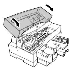
$10 \quad \text{After you close the top cover, the printer should automatically start cleaning the printer heads.}$
