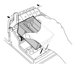
$10 \quad \mbox{Firmly press down the left lock lever to lock the colour BJ Cartridge in place.}$
