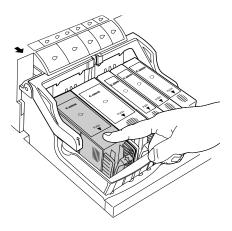
Check all the installed BCI ink tanks and make sure they are installed in the correct slots.
