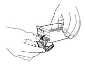
Insert the Color BJ Cartridge BC-82 Photo in the left cartridge holder.
