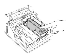
Pick up the Ink Tank BCI-8M (Magenta) and remove the shrink-wrap and orange protective cap (see Step 2 above).
