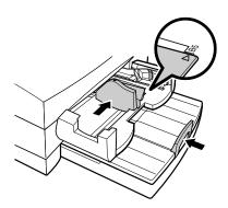
■ If the upper paper cassette is not extended, pull out the paper output tray and push in the paper output tray extension.
