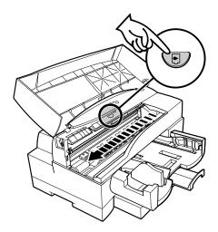
Remove the empty ink tank from the BJ Cartridge. Push in on the plastic lock on the ink tank to release it then lift it up out of the BJ Cartridge.
