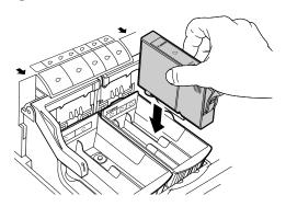
Press down on the top of the ink tank until it locks into place.
