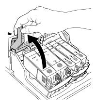
5 Lift the entire BJ Cartridge (print head and ink tanks together) out of the cartridge holder and set it aside.
