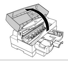
Press the **REPLACE** button. The cartridge holder moves to the left side of the printer.
