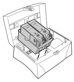
Make sure the BJ Cartridge is snug and seated correctly in the container. Then close the lid of the container and shut it completely.
