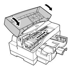
After you close the top cover, the printer should automatically start cleaning the print heads.
