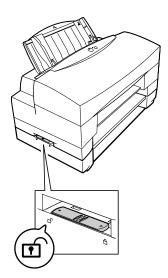
9 With two people on either side of the printer, raise the printer straight up to separate it from the optional paper cassette base.
