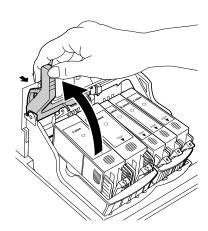
$\label{eq:first-state} 5 \quad \text{Lift the entire BJ Cartridge (print head and ink tanks together) out of the cartridge holder.}$
