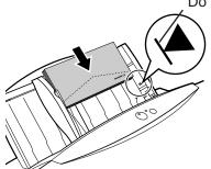
6 Slide the paper guide on the sheet feeder until it reaches the left edge of the stack.
