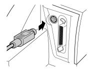
${\footnotesize 3} \quad {\footnotesize \text{Connect the other end of the printer cable to the printer port on the} \\ \quad {\footnotesize \text{Macintosh computer.}}$
