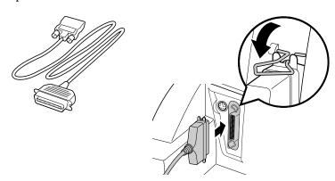
3 Connect the other end of the printer cable to the parallel connector on your computer. Fasten the clips or screws of the connector to secure the connection.
