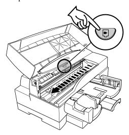
**A** Raise the cartridge lock lever on the left side of the cartridge holder.
