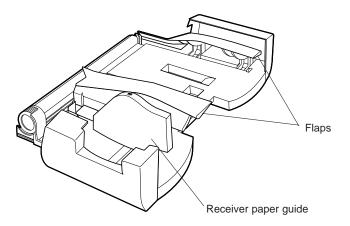
While holding the paper output receiver at a slight angle, insert it into the slot ① above the paper cassette and lower it ② gently as you slide it into the printer.
