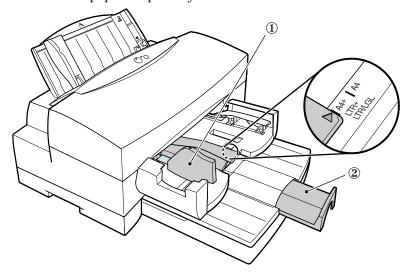
3 Check both the paper output receiver and the paper cassette and make sure that they are inserted completely into the printer.
