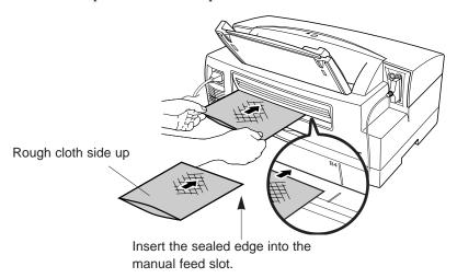
Hold the sheet in place for about 2 or 3 seconds. Wait for the printer to grab the sheet, then release it.
