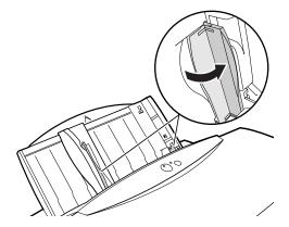
3 Make sure all the envelopes are pointing in the same direction and that no flaps are overlapping. With the flap sides down and the tops of the envelopes pointing down, insert the stack of envelopes into the sheet feeder.
