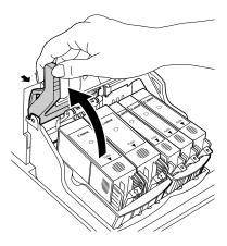
$\label{eq:continuous} 5 \quad \text{Lift the entire BJ Cartridge (print head and ink tanks together) out of the cartridge holder.}$
