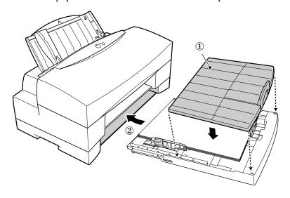
Press the paper cassette completely into the printer until it stops and locks in place.
