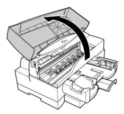
$\label{eq:controller} 3 \quad \text{Press the REPLACE} \text{ button near the centre of the printer.} \text{ The cartridge holder moves to the left side of the printer.}$
