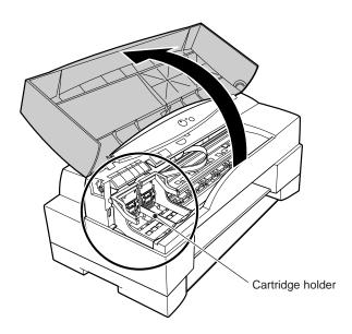
4 On both sides of the cartridge holder, raise both cartridge lock levers to their upright positions until they stop.
