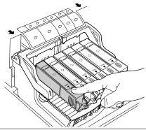
6 Check the ink tanks you just installed and make sure they are installed in the correct slots. Press down on each each ink tank to make sure that it is locked in place.
