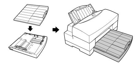
Adjust the length of the paper cassette for the length of the paper you are going to load.
