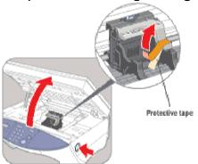
IMPORTANT: Remove the tape on the printhead holder lever.
