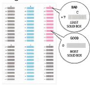
For the A Column printed pattern, use the \* the \* the \* to scroll to the value for the most solid box in the column.
