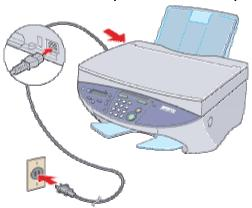
2. If the F30 MFP does not power up when plugged in, press the ON/OFF button to turn it on.
