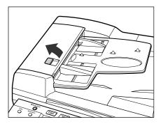
**2** Clean the rollers (total of two places), separator, and transparent plastic plate inside the feeder cover, with a cloth slightly dampened with water.
