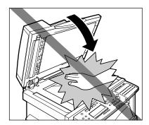
Do not press down hard on the feeder/platen glass cover when using the platen glass to make copies of thick books, etc. Doing so may damage the platen glass and result in personal injury.
