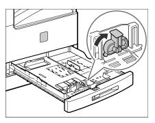
Lower the lock lever to the left to lock the side guide.
