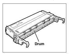
**8** While holding the toner cartridge with both hands, align both sides of the cartridge with the guiding grooves on the machine and insert the cartridge horizontally as far as it will go.
