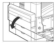
**3** Pull out the left cover of the stack bypass.
