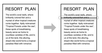
Follow the procedure described below to clean the original scanning area of the feeder.
