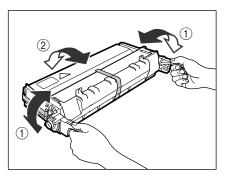
6 Place the toner cartridge on a flat stable surface, and hold the cartridge with one hand while removing the seal by pulling it out with the other hand.
