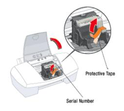
5. Write down the serial number located to the right of the printhead. You will need this later to register the product.
