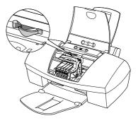
For regular paper and other media with a left position in the table (see "Load Limit and Paper Thickness Lever Position" on page 4).
