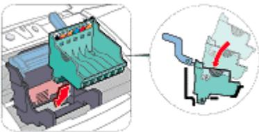
Lower the blue lock lever and gently press it down until you hear it lock into place.
