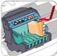
4. Insert the remaining five ink tanks into their assigned slots.
