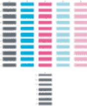
5. For each color on the test printout, enter the number in the Print Head Alignment window that corresponds with the smoothest looking test pattern.
