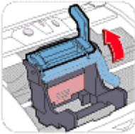
4. Gently set the printhead into the holder. The printhead will rest at a slight angle. Do not press it down.
