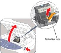
IMPORTANT: Remove the tape on the printhead holder lever.
