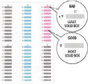
For the A Column printed pattern, use the see seekey to scroll to the value for the most solid box in the column.
