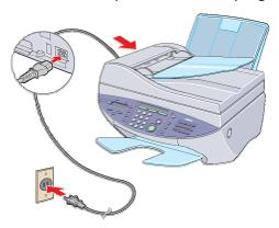
3. If the F50 MFP does not power up when plugged in, press the ON/OFF button to turn it on.
