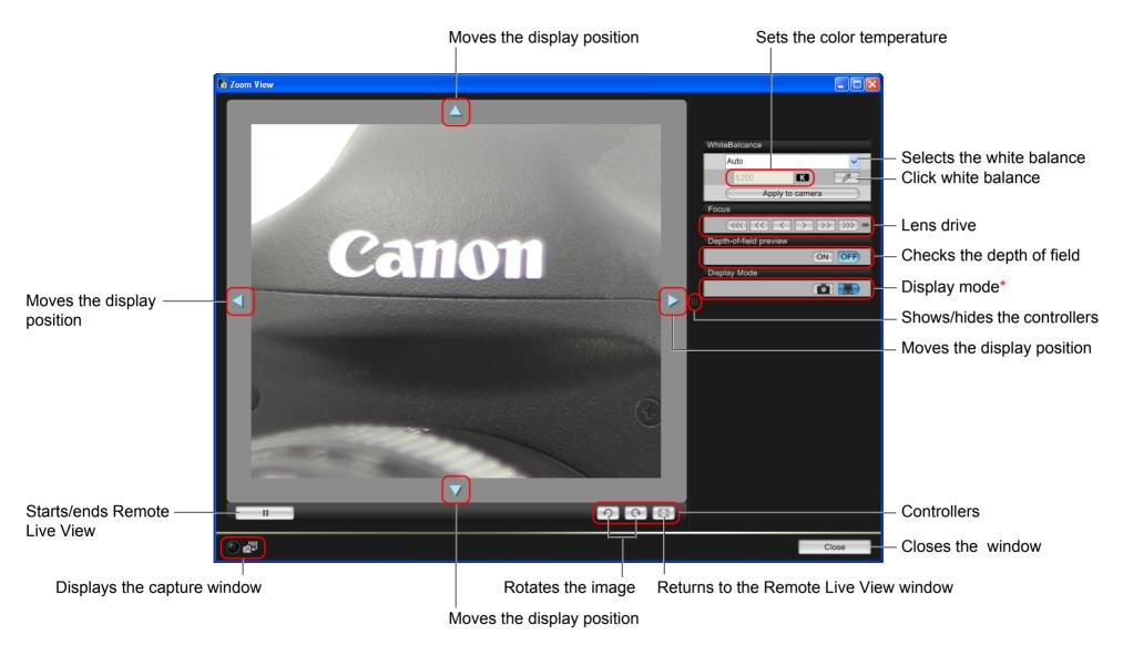
\* To focus while viewing on your camera's LCD monitor, click the [ button; to focus while viewing on your computer, click the [ button.
