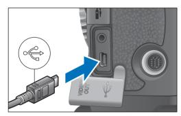
Connect with the < → > mark on the plug facing the front of the camera. 4 Attach the cable protector and fix it with the fixing screw.
