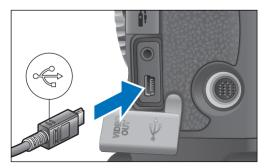
Connect with the < → > mark on the plug facing the front of the camera. Attach the cable protector and fix it with the fixing screw.
