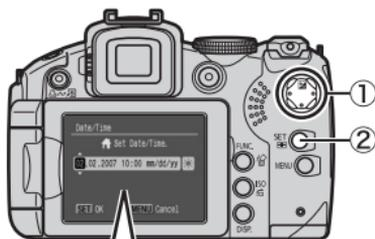
3. Confirm that the correct time is displayed and press the SET button (③).
