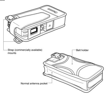
Water and dust resistance is further improved by using the WFT-E1A inside the supplied case. Under extreme operating conditions, insert the WFT-E1A into the supplied case during usage.
