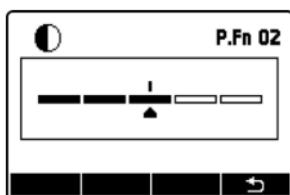
You can adjust the contrast of the LCD panel in 5 levels.
