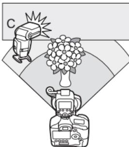
This section describes multiple flash shooting where slave C is added to flash tubes A and B.
