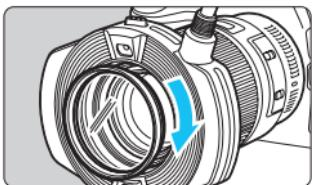
A commercially-available filter can be used during flash shooting. A filter can be attached, using the two procedures described below. Filters may not be used together with some macro lenses.
