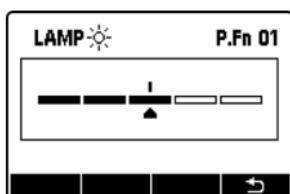
You can adjust the brightness of the focusing lamp in 5 levels.
