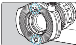
Press the <LAMP> button to light the focusing lamp for 20 sec., making focusing easier. Press the button again to turn off the lamp.
