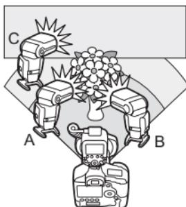
When C.Fn-15 is set to 1 (p.63), multiple flash shooting can be performed not only with slave C but also with slave A and B. For an outline of controlling flash, see "Slave Group Control" on page 46. Multiple flash shooting can be performed with flash tubes A and B as well as the slave unit(s) firing at the same output, or with only slave A or B added, regardless of the slave's firing group settings (p.54).
