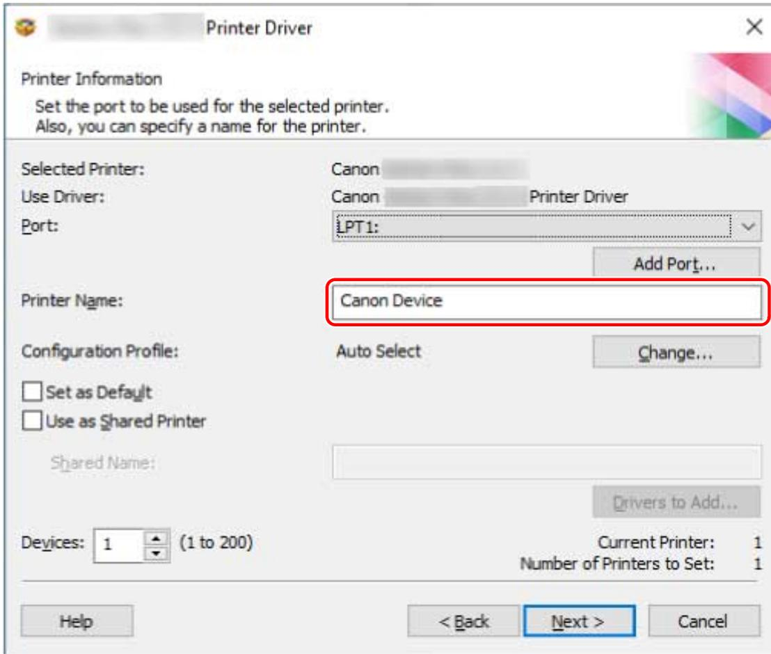
**9 If necessary, change the number of devices to be installed in [Devices] → click [Next].**
