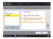
You can now specify settings to scan and then email/fax documents using a mobile device. When <Authenticate with PIN Code for Scan Jobs> is set to <On>, you must enter the PIN shown on this machine during job execution.
