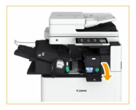
2 Turn the green knob to feed the jammed paper to the outlet of the puncher unit.
