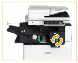
**3** If paper comes out of the outlet of the puncher unit, gently pull the paper out in the direction of the arrow.
