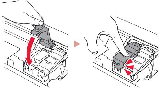
6 Repeat steps 2 to 5 and install the Black FINE cartridge as well, on the right-hand side.
