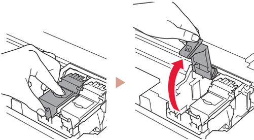
3 Remove the Color FINE cartridge from the container and remove the protective tape.
