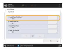
In situations such as direct printing where you cannot specify the paper source, you can now preset which paper source will be used beforehand. Set this to <Auto> to automatically switch to a paper source that matches the size and type of paper to be used for printing.
